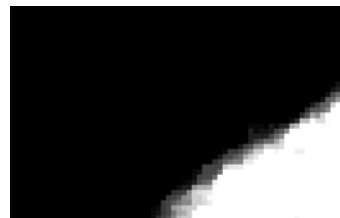
Figure 139. After T_Median has been applied with Radius= 1. Note the single pixel noise has gone.
