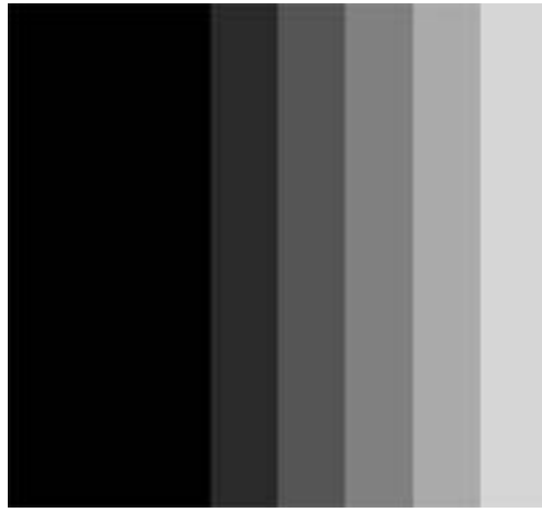
Figure 242. With Clip Min=21.74 and Clip Max=87.25 the three bottom bands have been clipped to black and the two brightest bands and been clipped to white.
