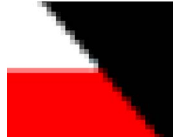
Figure 237. Wide Interpolation. Weighted interpolation over several lines.
